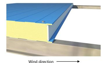
Proceed with the installation taking care to verify the perfect uprightness of the panel using temporary clamps
